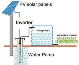
Ideally in some regions the storage would be 3-5 days of water demand. In practice some Installed tanks do not have sufficient capacity and are smaller than a days demand leaving the tank empty at the end of the day. This is due to a mismatch between the sizing, pump capacity and the demand profile during the day.
